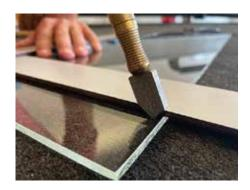
**CUTTING**ALL GLASS THICKNESSES FROM 3 TO 25 MM
